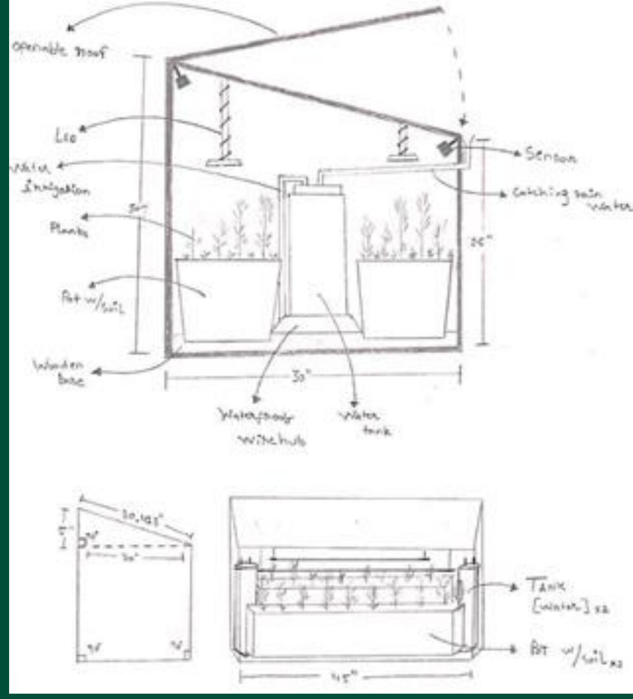
Figure 2: Smart Greenhouse Design-2
