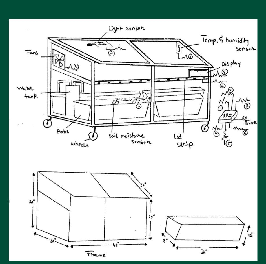
Figure 1: Smart Greenhouse design-1
